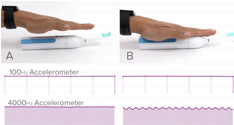
Viband: High-fidelity bio-acoustic sensing using commodity smartwatch accelerometers
