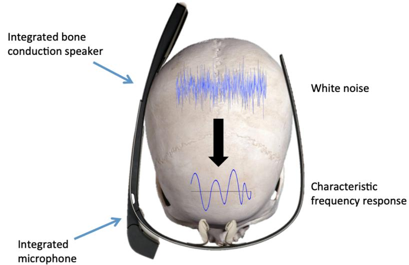
SkullConduct: Biometric User Identification on Eyewear Computers Using Bone Conduction Through the Skull
