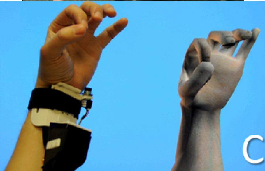
Digits: freehand 3D interactions anywhere using a wrist-worn gloveless sensor
